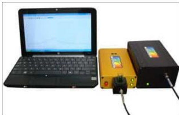
Figure 2. StellarNet BLACK-Comet spectrometer including computer setup (StellarNet, 2018).
