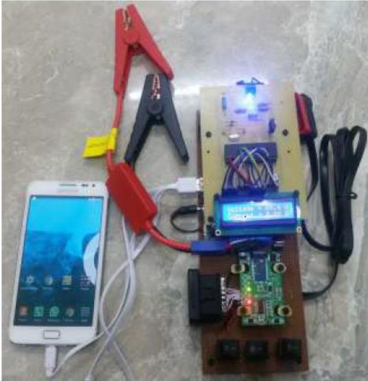
Figure 3: The results of OBDII interface connected for malfunctioning
