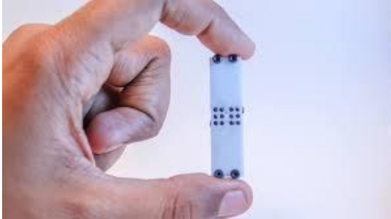
Figure 11. Refreshable Braille pins [10]
