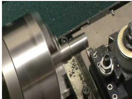
Figure 2: Turning operation on mild steel (Lathe Turning Steel, 2019)
